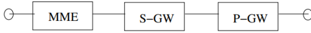
Fig. 4: Structural model of element connection of MME, S-GW and P-GW in terms of reliability
