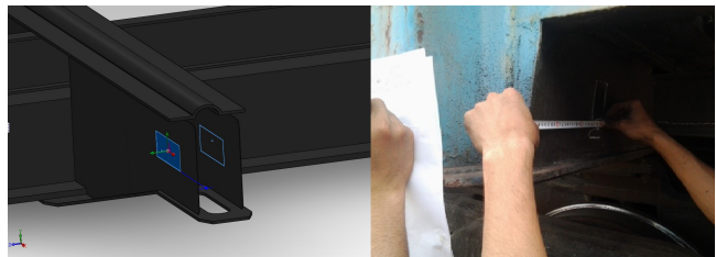
Fig. 3: Measurement of the pivot beam of the frame of the weighing wagon 640-VPV-277
