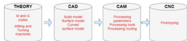
Fig. 4: CAD/CAM/CNC integrated teaching process
