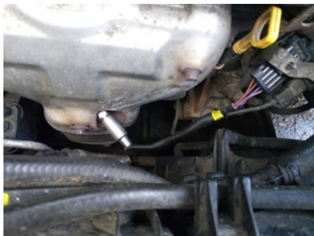
Fig. 6: Oxygen sensor adapter installed on the car
