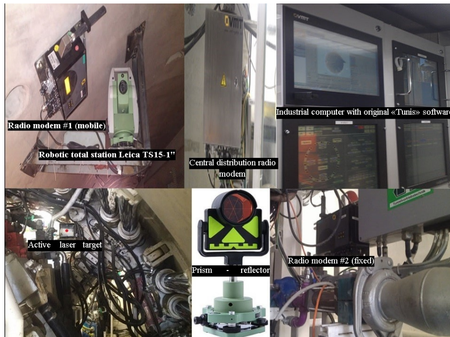
Fig. 1: Technical means of navigation equipment of the SLS-SL system by VMT GmbH
