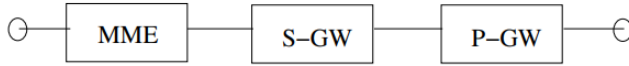
Fig. 4: Structural model of element connection of MME, S-GW and P-GW in terms of reliability
