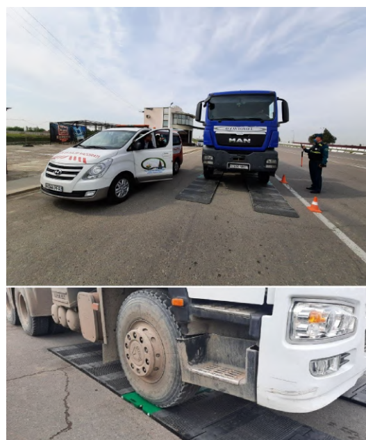
Fig. 11: Process of weighing of cargo transport vehicles at the MWDCS
