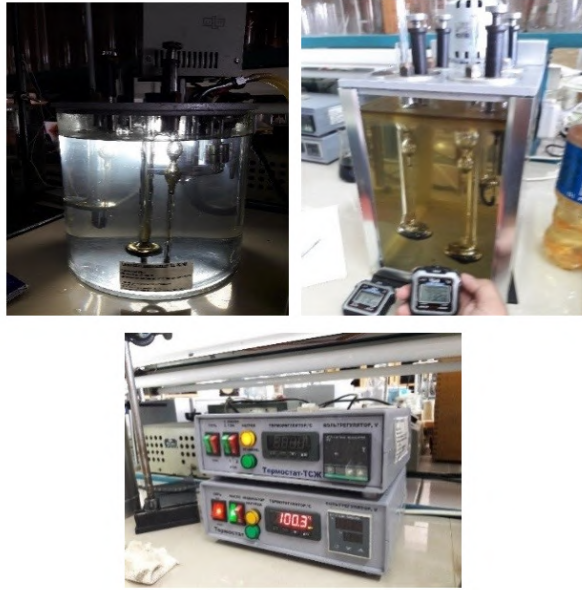
Fig. 3: The process of determining the viscosity of engine oil at temperatures of 40 and 100°C.
