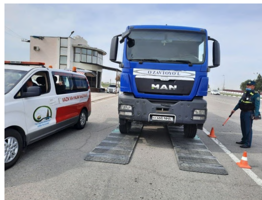
Fig. 10: Process of weighing of cargo transport vehicles at the MWDCS
