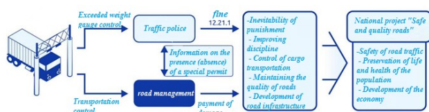
Fig. 1: The system of weight and dimension control of vehicles (on the example of the Russian Federation)
